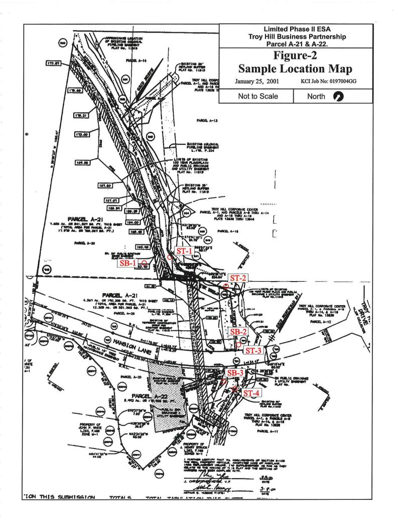
The three (3) shallow subsurface soil samples, designated SB-1 through SB-3, were collected from locations where KCI observed dumped drums, chemical containers, and other debris. KCI's purpose in collecting these samples was to investigate the possibility of soil contamination resulting from the debris.
